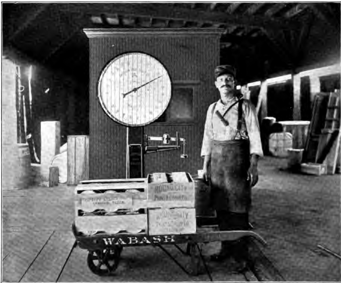
This shows the American Kron Automatic Dial Scale in operation on the Wabash R. R.
